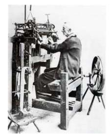
probably dates from the late 19th century, shows a knitter working a typical frame. On the right is a bobbin winder, adapted from an old spinning wheel.
